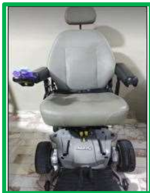
Figure 3. Electric wheelchair with the proposed adaptation.
