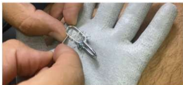
Image 7. Shows the links being sewn onto the gloves.
